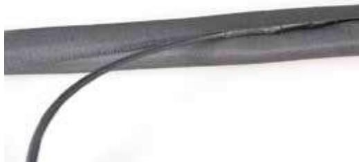
ShrinkTech's SCW self-closing wrap is a non-expandable sleeving woven from monofilament weft and multifilament warp polyester yarns. It provides a lightweight, cost-effective and tough solution for the protection of a wide range of components. Its inherent flexibility allows it to bend, coil and conform to irregular shapes, while its open design allows it to be installed on completed assemblies.
