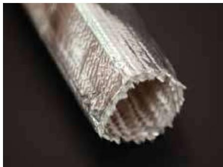
STF-ALU is a flexible sleeve made of fiberglass braid covered with an aluminum foil. The tube offers a continuous working temperature of -40°C up to +220°C. Its smooth and reflective outer surface provides a very reflective barrier to radiant heat. Used within the automotive sector.
