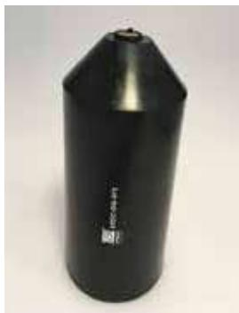
De Gassing is heat shrinkable end caps, supplied with relief valve, are used for sealing high voltage cable ( up to 33kV) to release the constantly evolving gas generated inside the cable during transportation and storage in hot climate conditions..
